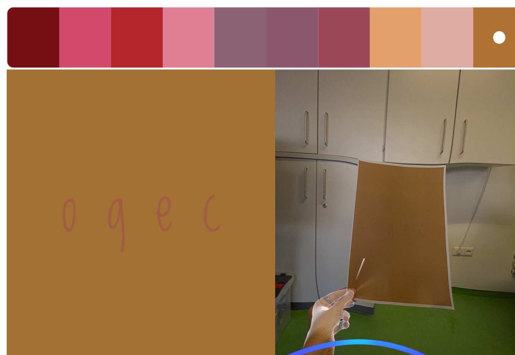
A comparison of contrast perception between a physical image (left) and its view through a virtual see-through device (right) from the surgical colour palette (top).
